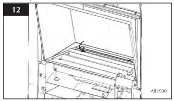
7.3 Secure the panel using the two upper brackets and the pozidrive screws, Diagram 13. Use only the rearmost hole in the retaining bracket on each side.
